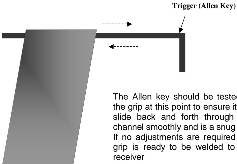
The Allen key should be tested in the grip at this point to ensure it will slide back and forth through the channel smoothly and is a snug fit. If no adjustments are required the grip is ready to be welded to the receiver
