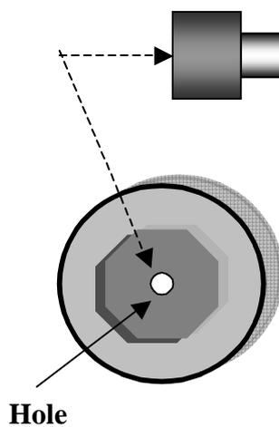
A 2mm diameter hole is drilled in the centre of the bolt head to a depth of  $\frac{5}{8}$ ". The firing pin is a section of 2mm diameter drill shank 25mm in length. The pin should protrude 1 to 1.5 mm from the face of the bolt head when inserted. The pin is retained using bearing adhesive.
