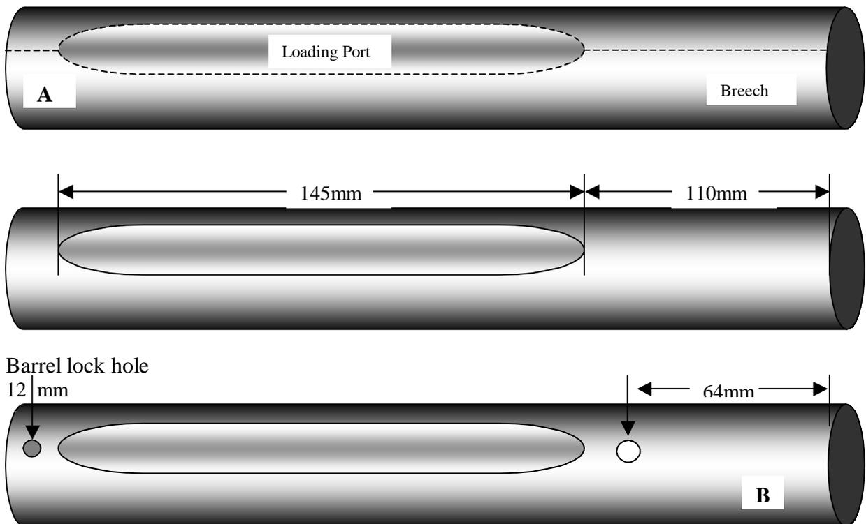
The next step is to drill two holes. The two holes will accept the 'sear spring' and 'barrel lock spring' in due course. The sear spring hole is drilled 64mm from the breech end, and is 6.5mm in diameter.
