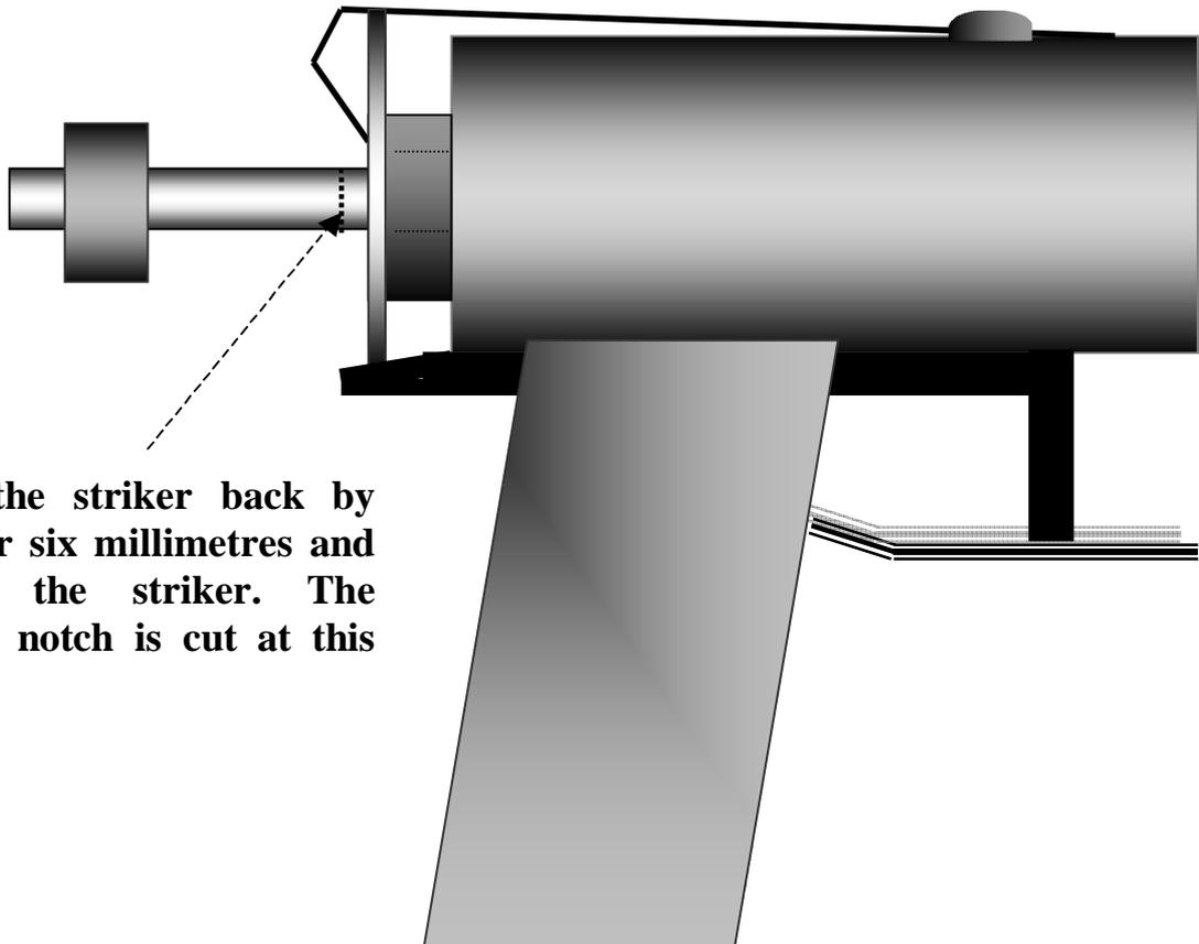
**Pull the striker back by five or six millimetres and mark the striker. The safety notch is cut at this point.**
