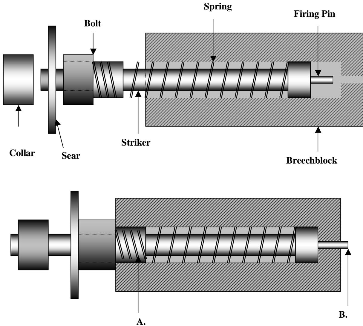
Screw in the retaining bolt 'A' and check all parts are moving smoothly.
