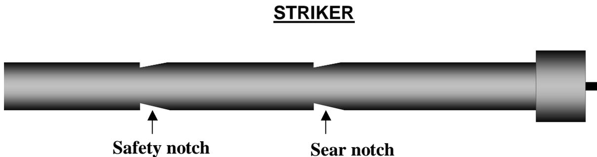
**With the notches cut, the striker can be re-fitted and the weapon is ready to test fire.**
