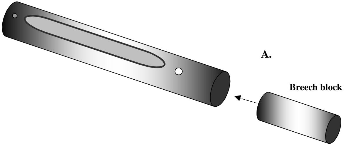
The breech block is inserted into the end of the receiver as shown in Figure 'A'. The block is pushed into the receiver until the end of the block is seated to a depth of 1/8", as shown in Figure 'B' below.
