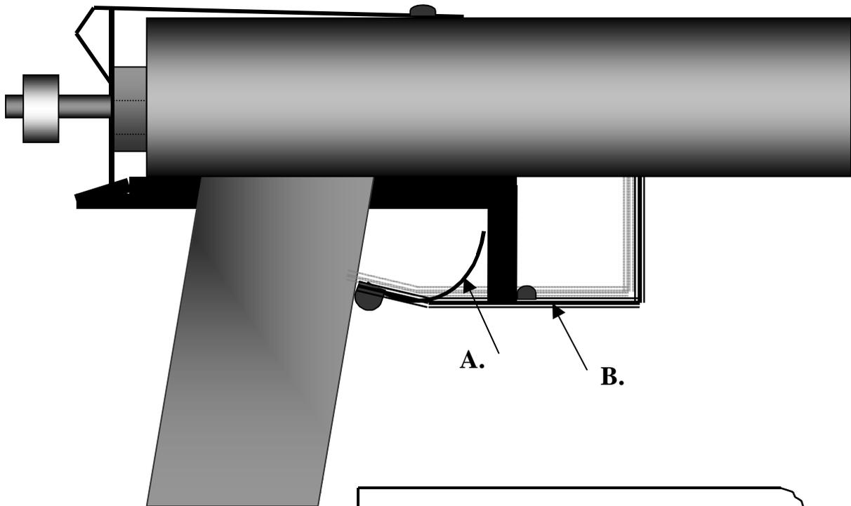
With the trigger stop screw fitted, the gap between the front of the grip and the rear of the trigger should be about 35mm.
