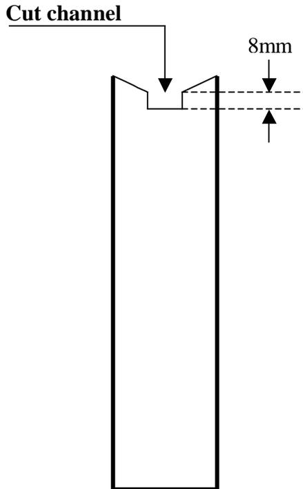
After cutting the curved groove across the top of the grip a square channel can now be cut to accept the trigger bar.
